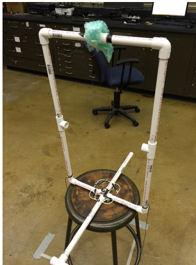
Figure 9.1: PVC rig used to constrain the motion of Crazyflie to just vertical
