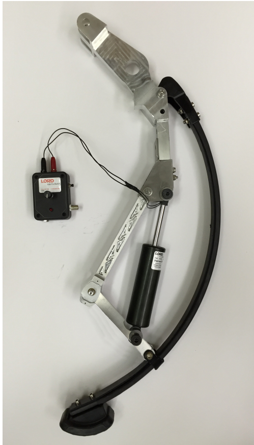
Figure 2.7: Picture of prototype built of HIL shin leg section
