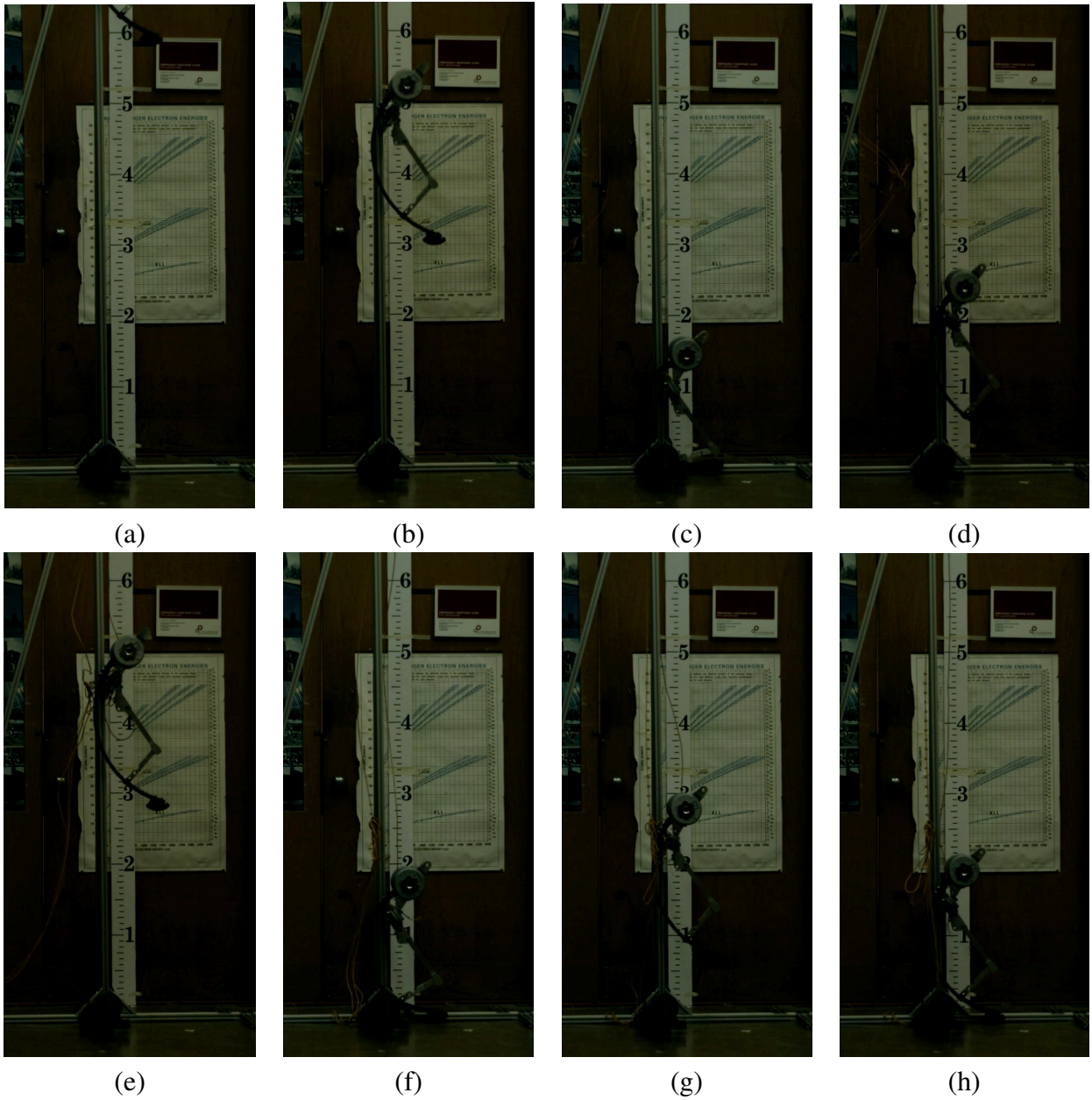
Figure 4.8: High speed video screenshot sequence of drop test set (1) from 6ft with 15kg payload mass. Leg bounced 3 times before coming to a rest with a max bounce height of 2ft 8in.
