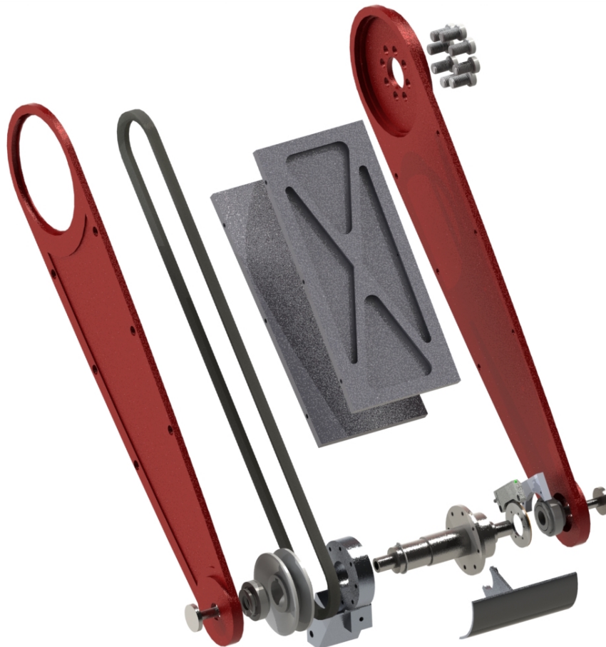
Figure 2.5: 3D CAD exploded view of HIL thigh leg section
